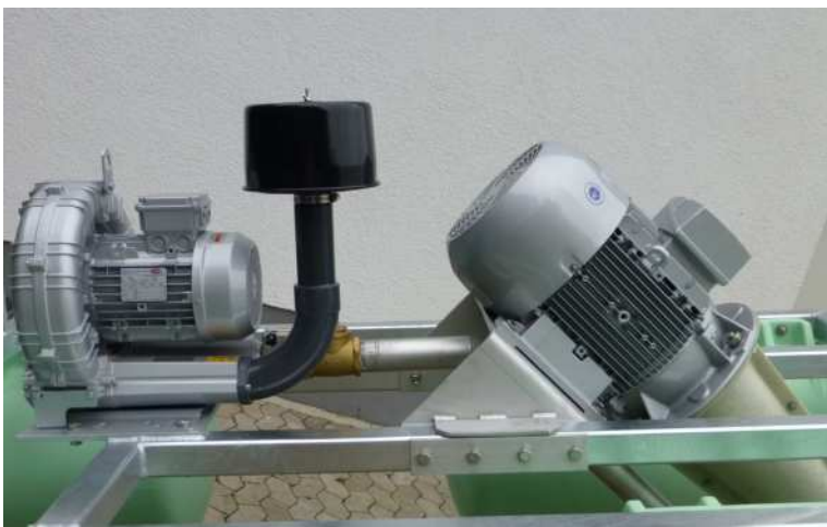
DUALSTAR: blower with air filter, silencer and non return valve
